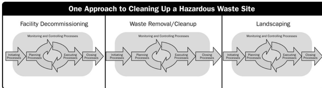
Figure 2-11. Example of a Three-Phase Project
